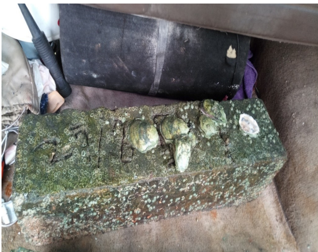
Figure 5: Beam buried in Lagoon water after 1 year.
