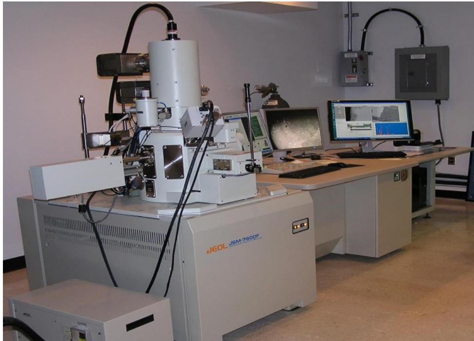
Figure 3: SEM complete system.
