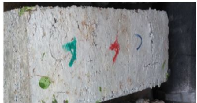
Figure 6: Beam buried in Fresh water after 1 year.
