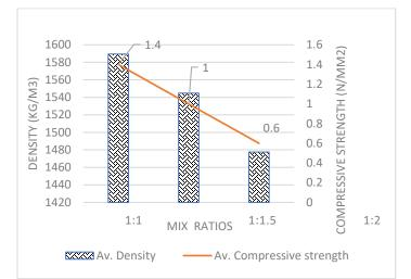
**Figure 5:** Relationship between density (kg/m<sup>3</sup>) against 21 days compressive strength (N/mm<sup>2</sup>) for sand-PET mix
