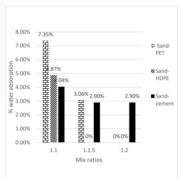
Figure 4: Relationship between % water absorption and mix ratios
