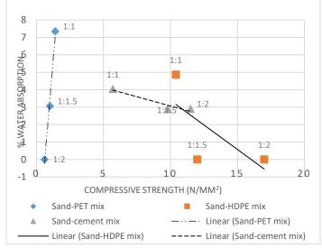
Figure 9: Relationship between % water absorption and compressive strengths for the various mix combination and proportions
