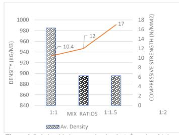
**Figure 6:** Relationship between density (kg/m<sup>3</sup>) against 21 days compressive strength (N/mm<sup>2</sup>) for sand-HDPE mix.
