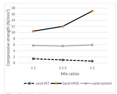
Figure 8: Relationship between compressive strengths and the mix ratios.
