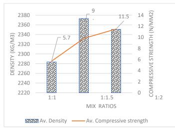
**Figure 7:** Relationship between density (kg/m<sup>3</sup>) against 21 days compressive strength (N/mm<sup>2</sup>) for sand-cement mix.
