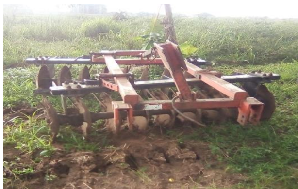
Figure 2: The Disc Harrow (Baldan Implementos Agricolas, Brazil) used in this Study
