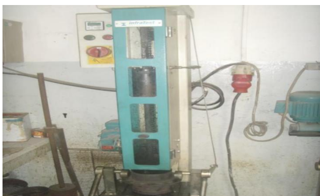
Figure 3: Sample of asphalt concrete in compaction mould
