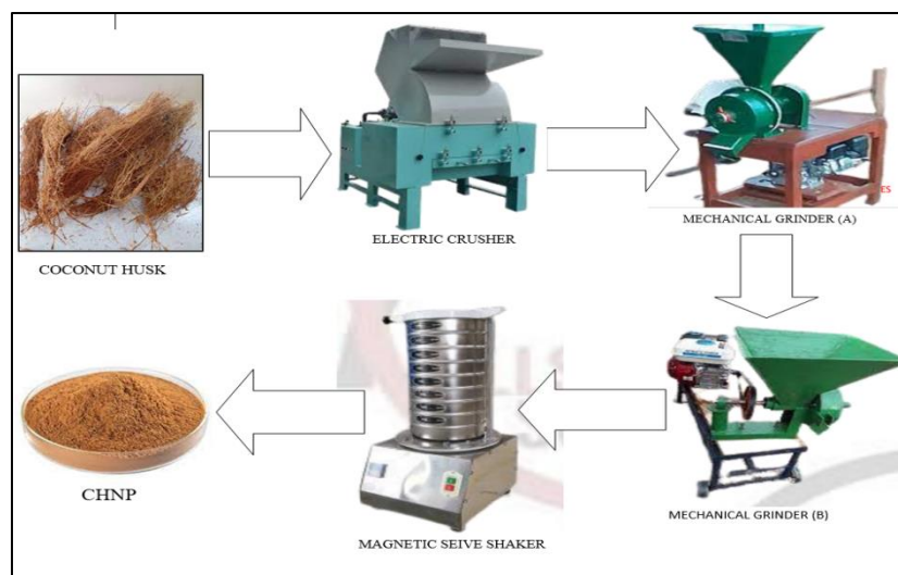
Figure 1: Coconut husk nano-sizing process
