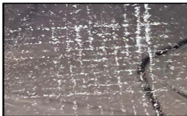
Plate 1: Photograph of the adhesion test tape of the sample
