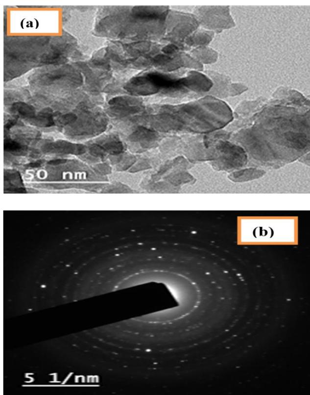
**Figure 5:** (a) HRTEM image of TiO<sub>2</sub> NPs, (b) Selected area electron diffraction (SAED) pattern
