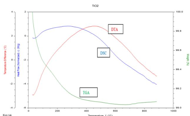
**Figure 6:** DTA-DSC and TGA of TiO<sub>2</sub> NPs
