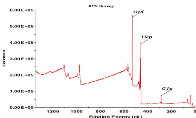
Figure 7: XPS full survey spectra of TiO<sub>2</sub> NPs
