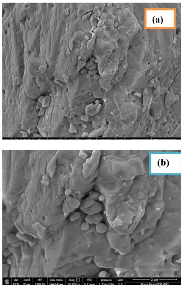
**Figure 4:** FE-SEM micrograph images of TiO<sub>2</sub> NPs at a) 25,000 $\times$  and b) 50,000 $\times$
