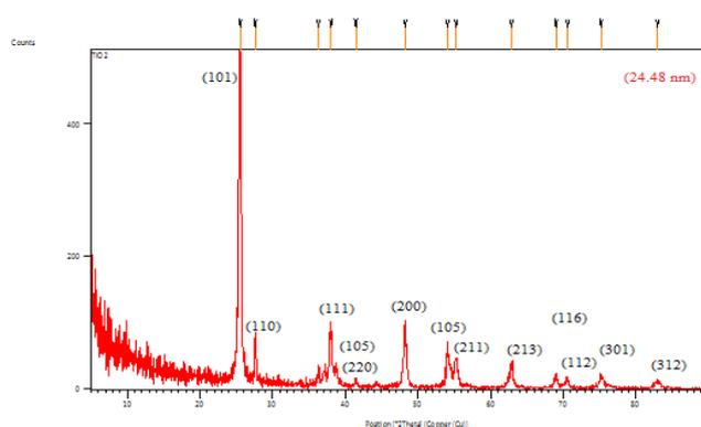
**Figure 2:** X-ray diffraction pattern of titanium dioxide nanoparticles (400 °C, 3 hours)
