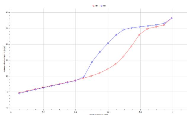
Figure 3(b): BET Adsorption-Desorption isotherm of TiO<sub>2</sub> NPs
