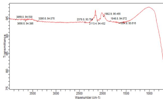
**Figure 1:** Analysis of titanium dioxide nanoparticles (TiO<sub>2</sub> NPs) using Fourier Transform Infrared (FTIR) spectroscopy
