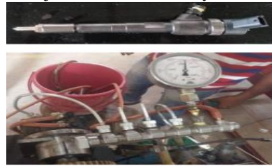
(d) Fuel IOP is recorded using a CRDI injector and a pressure gauge.
