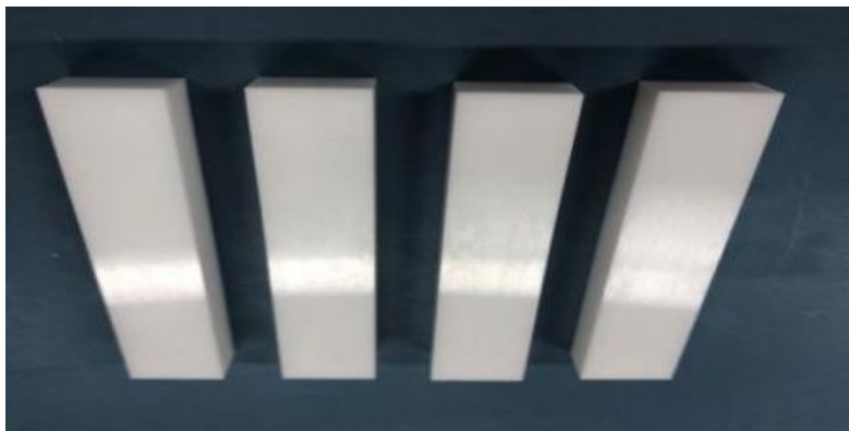
Figure 3: Machined specimen for hardness test
