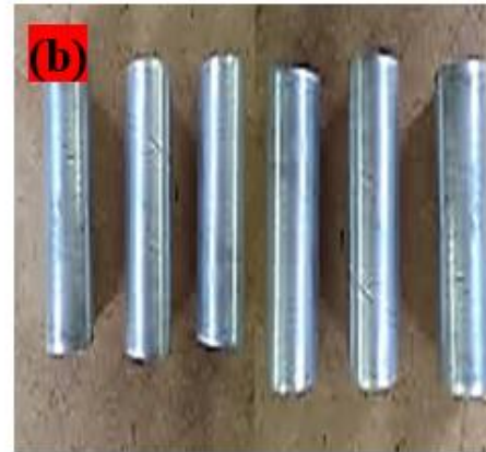
Figure 1: Aluminium 6063 sample (a) prior machining for extrusion (b) after machining for extrusion
