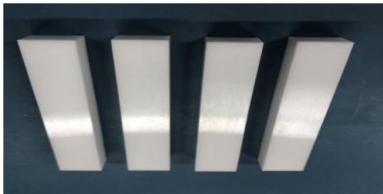
Figure 3: Machined specimen for hardness test
