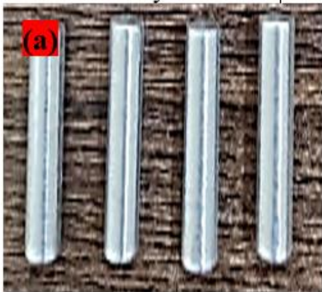
Figure 1: Aluminium 6063 sample (a) prior machining for extrusion (b) after machining for extrusion
