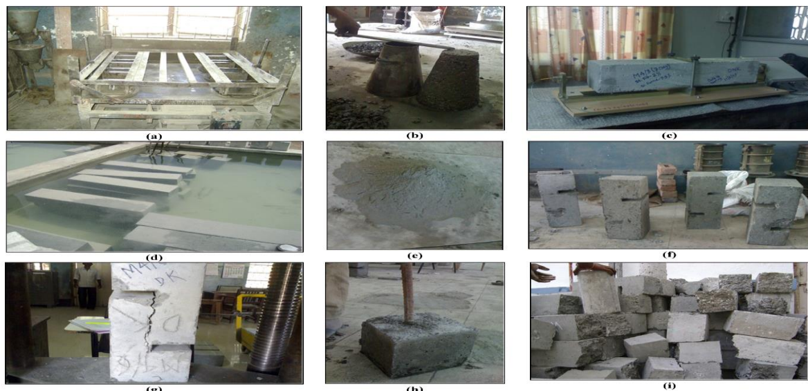
Figure 1: (a) Table vibrator arrangement in Laboratory for compaction; (b) Slump measurement; (c) Electrodynamic Test Setup for Longitudinal Frequency; (d) Curing of Specimen; (e) Dry Concrete Mix with Silica fume and Steel Fibers; (f) Shear Specimens; (g) Shear Test Set up After Failure; (h) Pull out Specimen Before Failure; and (i) Broken Specime.
