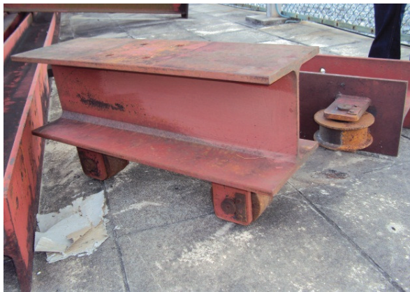
Figure 12: Part of clamp carriage showing rollers.
