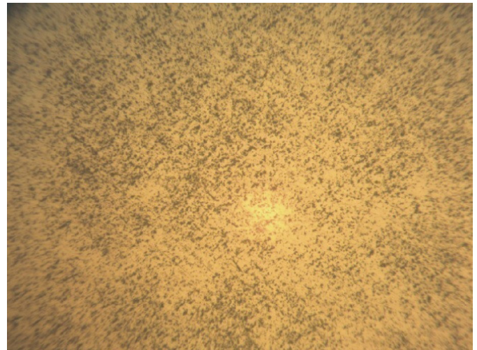
Figure 3: Micrograph of Al-12wt%Si + 0.05% S alloy casting (200x).
