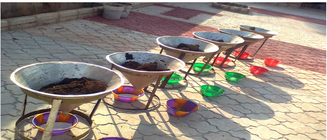
Plate 1: Experimental set-up for dewaterability of conditioned sludge
